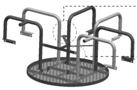
**Step 2**Assembly of the Link onto the 6 legs
